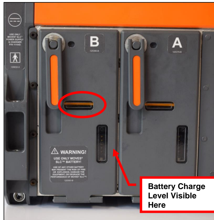
Figure 9-11: Visible Yellow Handle Indicates Battery Present
