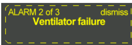
Figure 15-5: Latched Alarm Able To Be Dismissed
