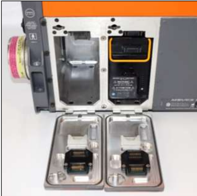
Figure 9-10: Battery Disconnected (compartment open)
