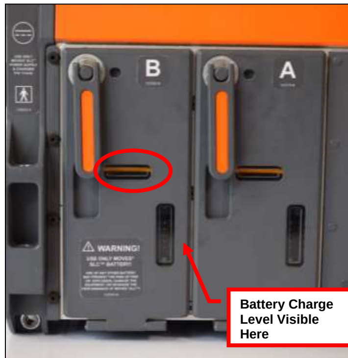
Figure 9-9: Visible Yellow Handle Indicates Battery Present
