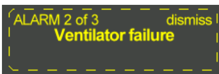
Figure 15-5: Latched Alarm Able To Be Dismissed
