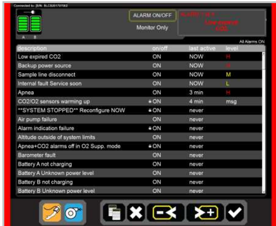
Figure 12-13: Red Bars Indicating High-Priority Alarm Active
