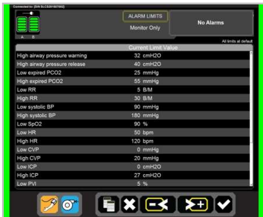
Figure 12-12: Green Bars Indicating No Alarms Active
