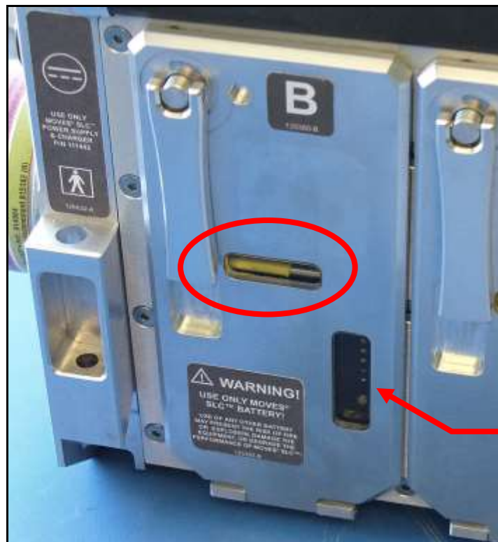
Figure 9-9: Visible Yellow Handle Indicates Battery Present
