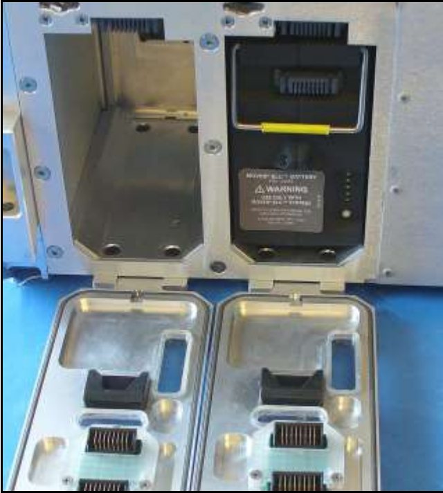
Figure 9-10: Battery Disconnected (compartment open)
