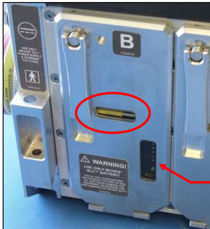
Figure 9-9: Visible Yellow Handle Indicates Battery Present
