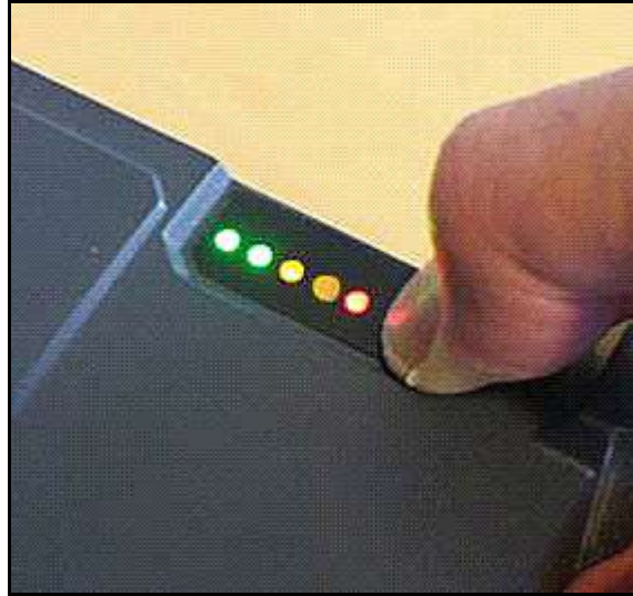
Figure 9-8: Condition Indicator Showing High Level Charge
