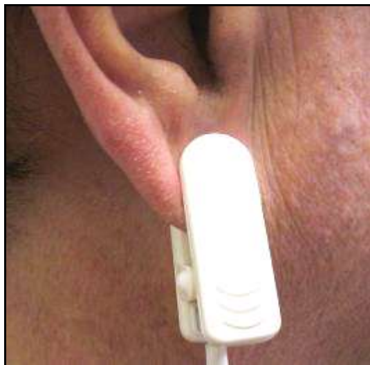
Figure 13-2: Correct Ear Lobe Sensor Placement
