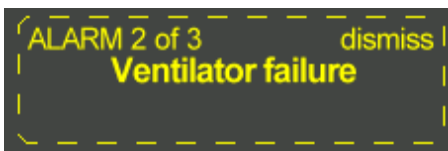
Figure 15-5: Latched Alarm Able To Be Dismissed
