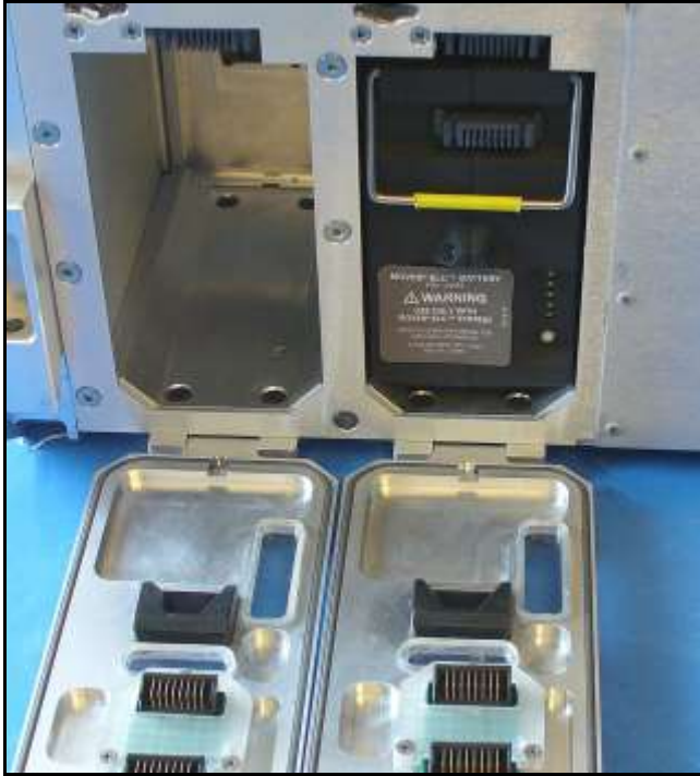
Figure 9-11: Battery Disconnected (compartment open)
