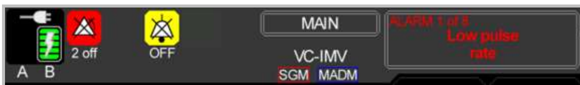
Figure 15-6: Status Bar Showing Safe Gas Mode Indicator When MADM™ Connected
