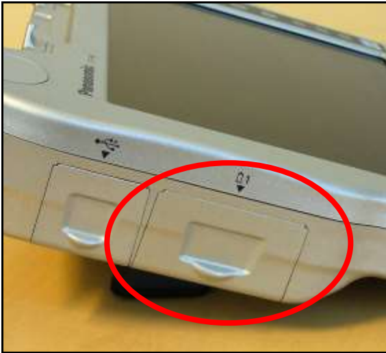
Figure 12-2: Battery Bay 1 on Left Side
