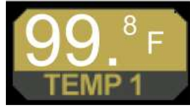
Figure 11-23: Inverted Display of Temperature (Alarm Condition)
