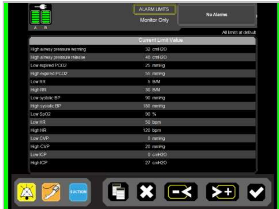
Figure 12-13: Green Bars Indicating No Alarms Active
