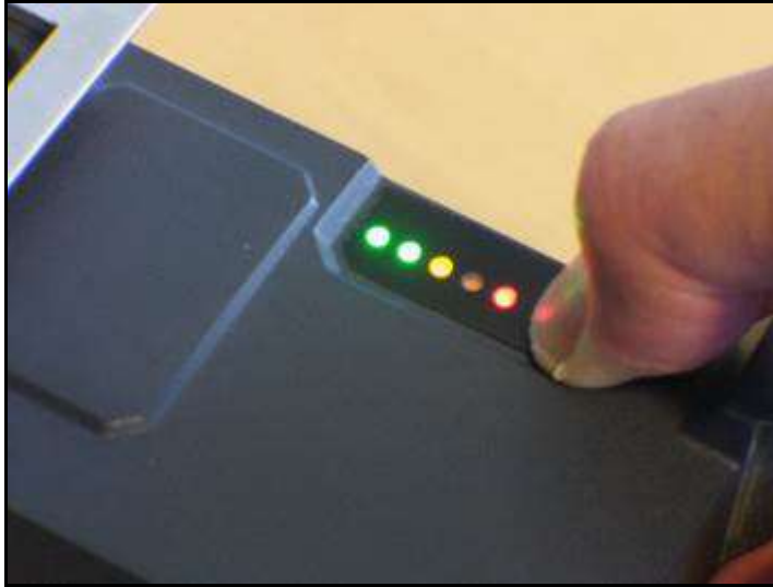
Figure 9-9: Condition Indicator Showing High Level Charge
