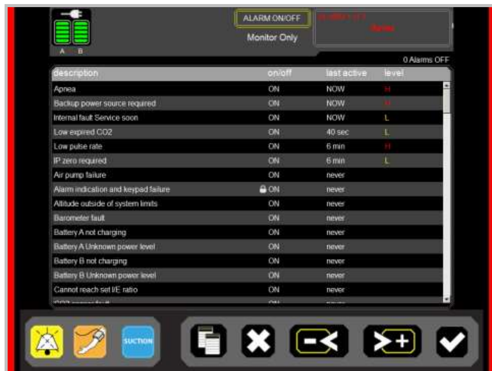
Figure 12-14: Red Bars Indicating High-Priority Alarm Active
