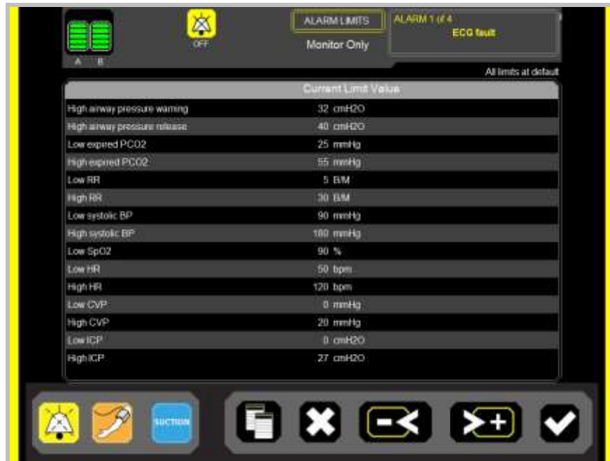
Figure 12-15: Yellow Bars Indicating Low or Medium Priority Alarm Active
