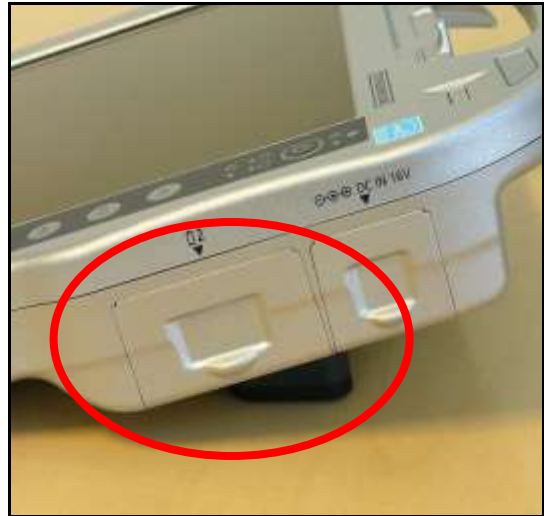
Figure 12-3: Battery Bay 2 on Right Side
