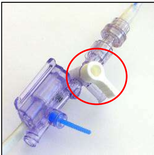
Figure 13-8: Transducer Stopcock in Running Position (Horizontal)
