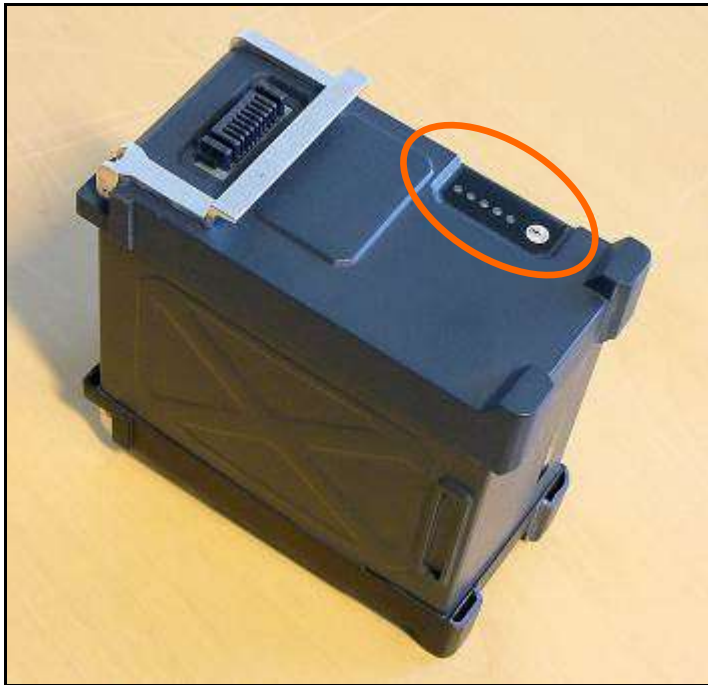
Figure 9-8: Battery with Condition Indicator Shown
