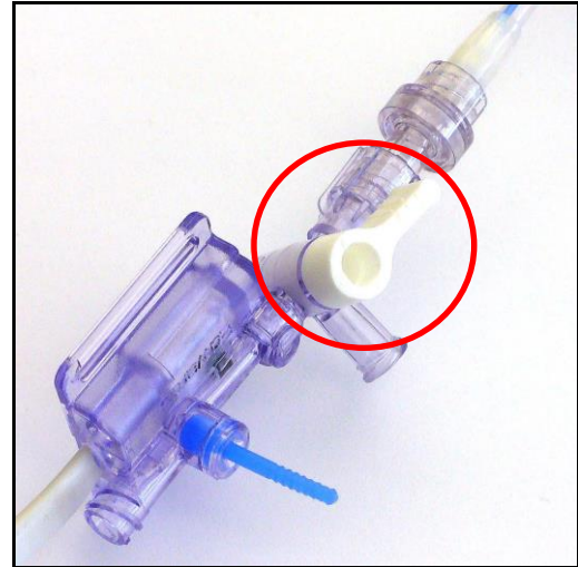
Figure 13-9: Transducer Stopcock in Open-to-Ambient-Air Position (Vertical) Zero Transducer
