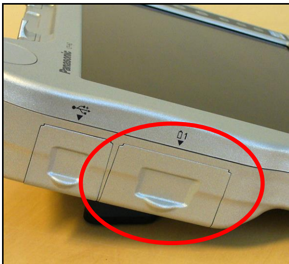
Figure 12-2: Battery Bay 1 on Left Side
