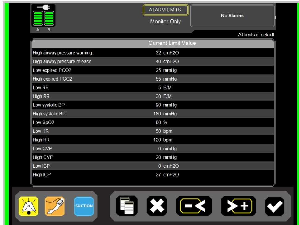
Figure 12-11: Green Bars Indicating No Alarms Active
