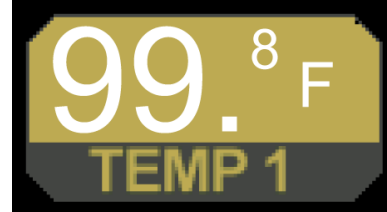
Figure 11-19: Inverted Display of Temperature (Alarm Condition)
