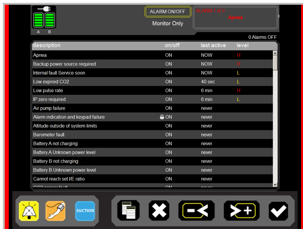
Figure 12-12: Red Bars Indicating High-Priority Alarm Active
