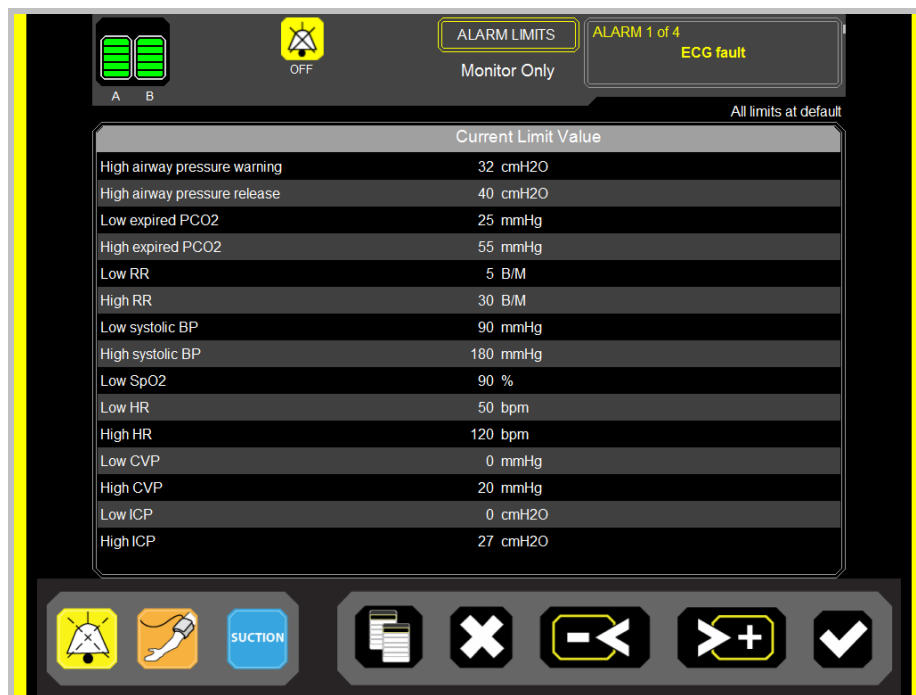
Figure 12-13: Yellow Bars Indicating Low or Medium Priority Alarm Active
