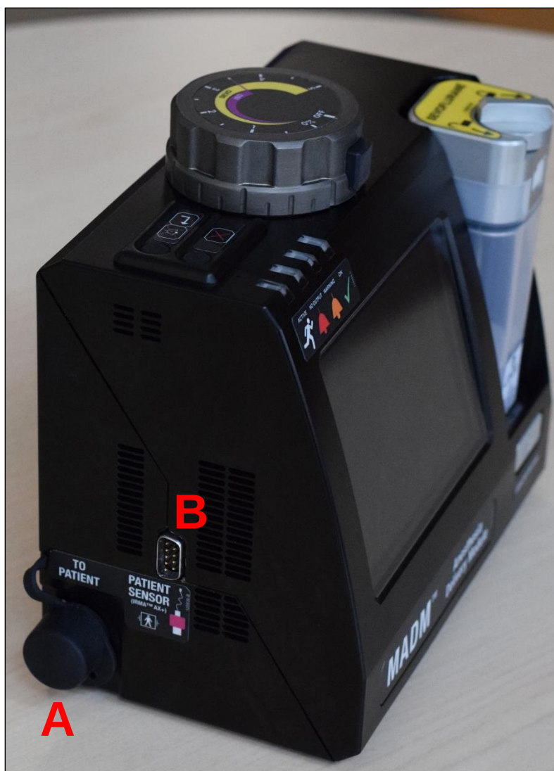
Figure 16: Left Side Connections
