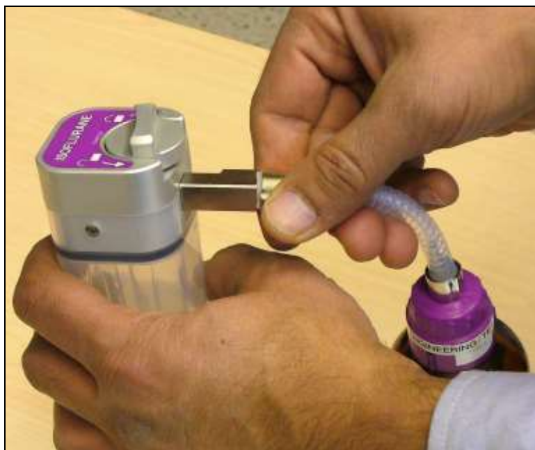
Figure 32: Insert the Rectangular Fitting
