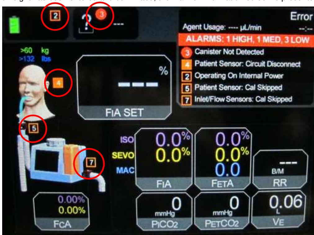
Figure 11: Information Screen – Showing Four Errors
