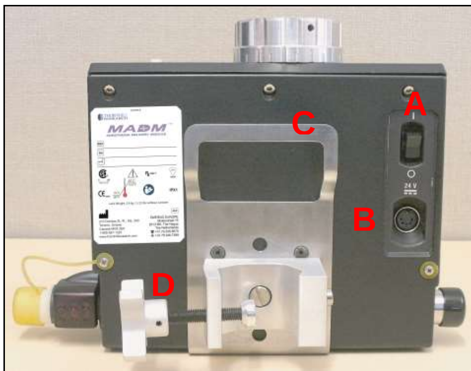
Figure 18: Rear Controls and Connections
