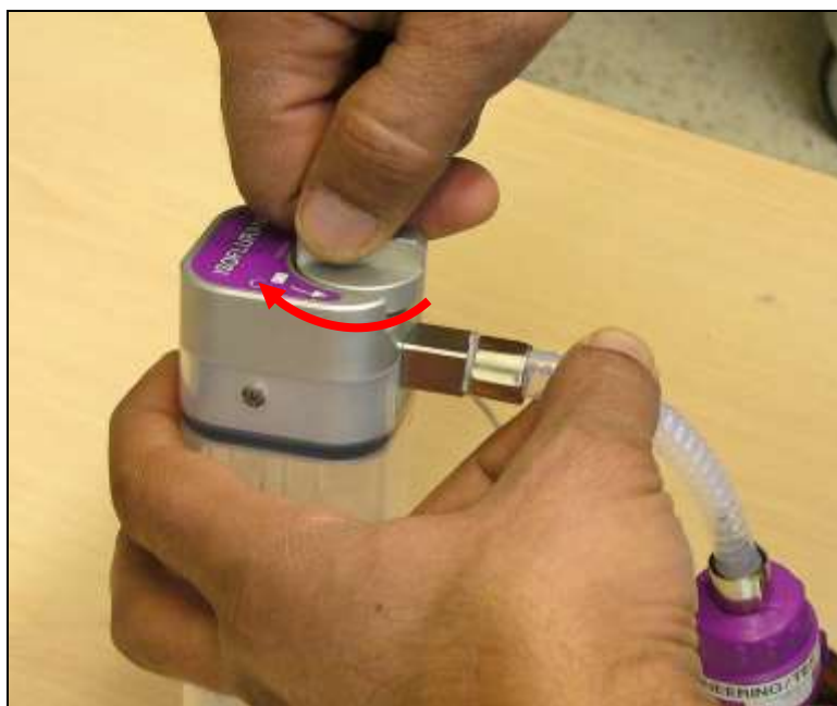
Figure 33: Turn Knob Clockwise to Secure
