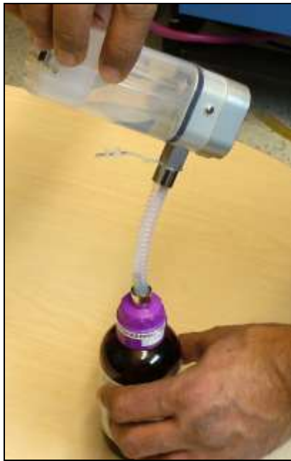
Figure 33: Raise Canister Above Bottle
