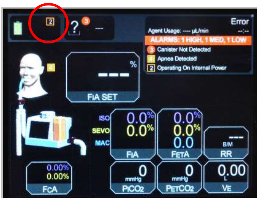
Figure 10: Information Screen – Three Alarms
