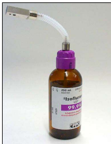
Figure 26: Bottle with Gooseneck Attached
