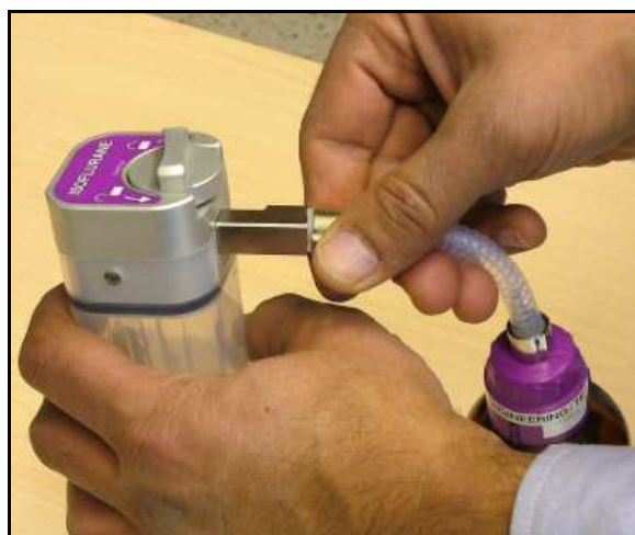
Figure 27: Gooseneck Fitted to Canister
