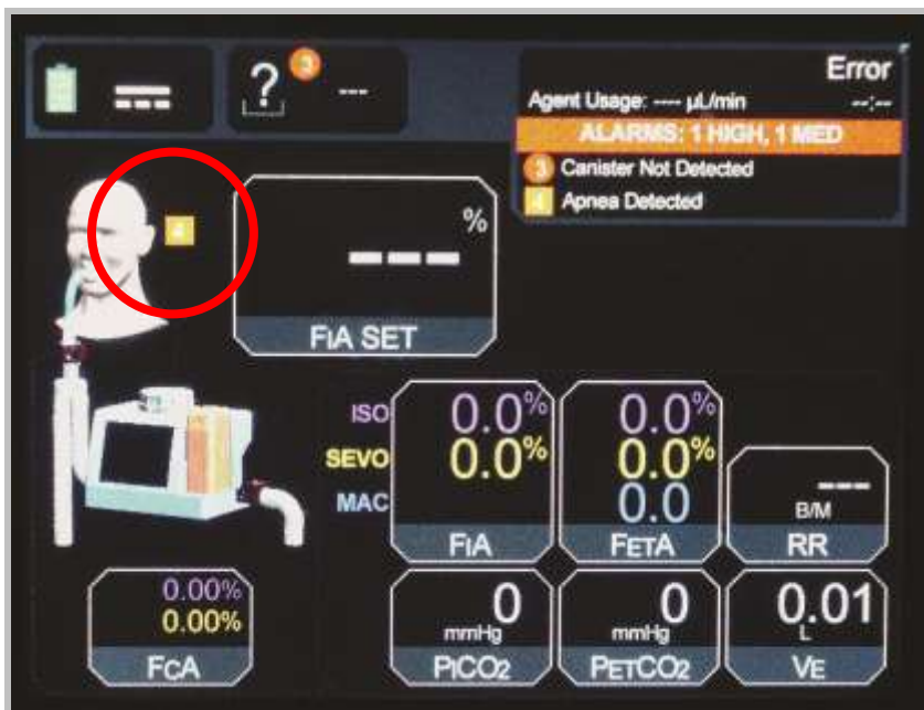
Figure 9: Information Screen – Two Alarms
