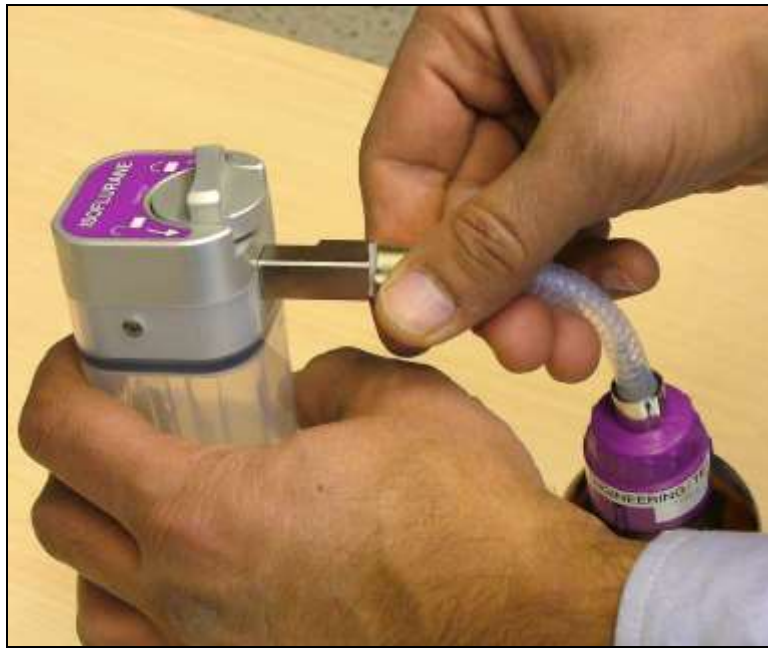
Figure 31: Insert the Rectangular Fitting
