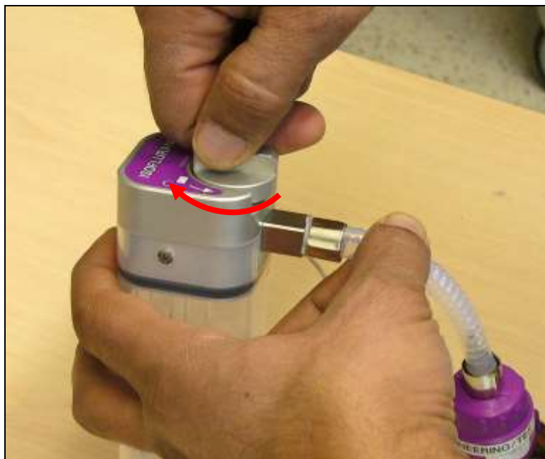
Figure 32: Turn Knob Clockwise to Secure
