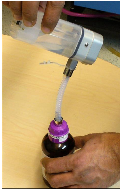
Figure 38: Raise Canister Above Bottle
