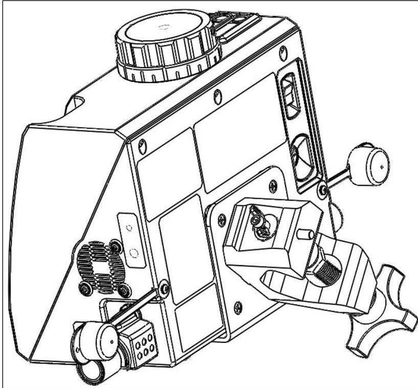
Figure 23: Clamp Mating to Mounting Bracket at 45-Degrees
