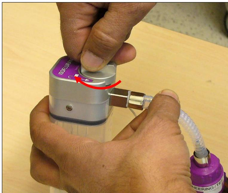
Figure 37: Turn Knob Clockwise to Secure
