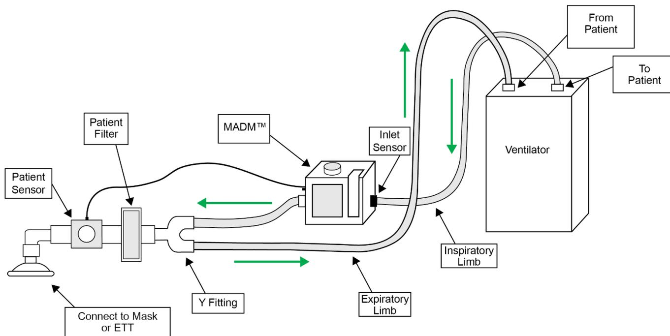
Figure 27: Closed Circuit with Ventilator Assembly Diagram
