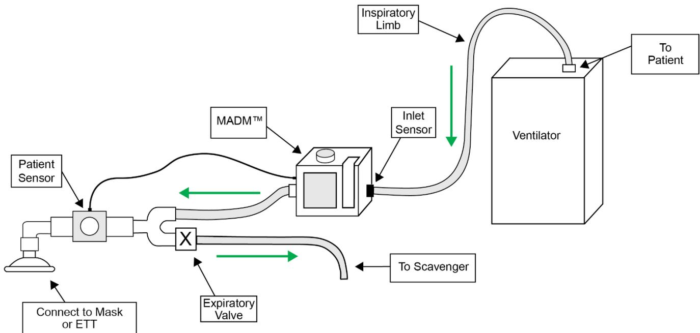
Figure 26: Open Circuit with Ventilator Assembly Diagram
