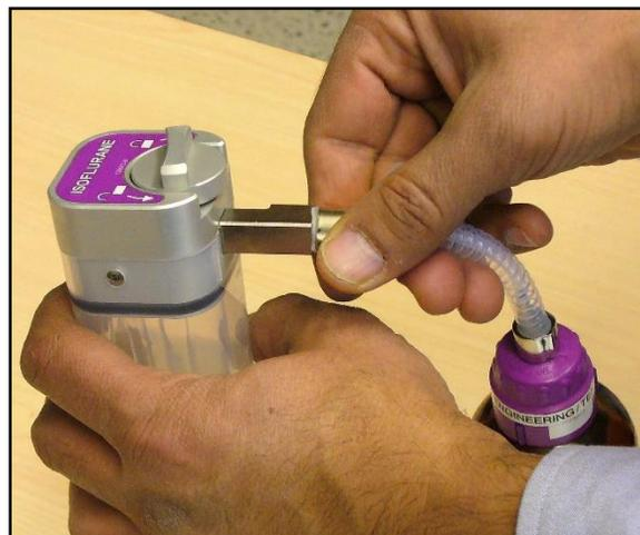
Figure 32: Gooseneck Fitted to Canister
