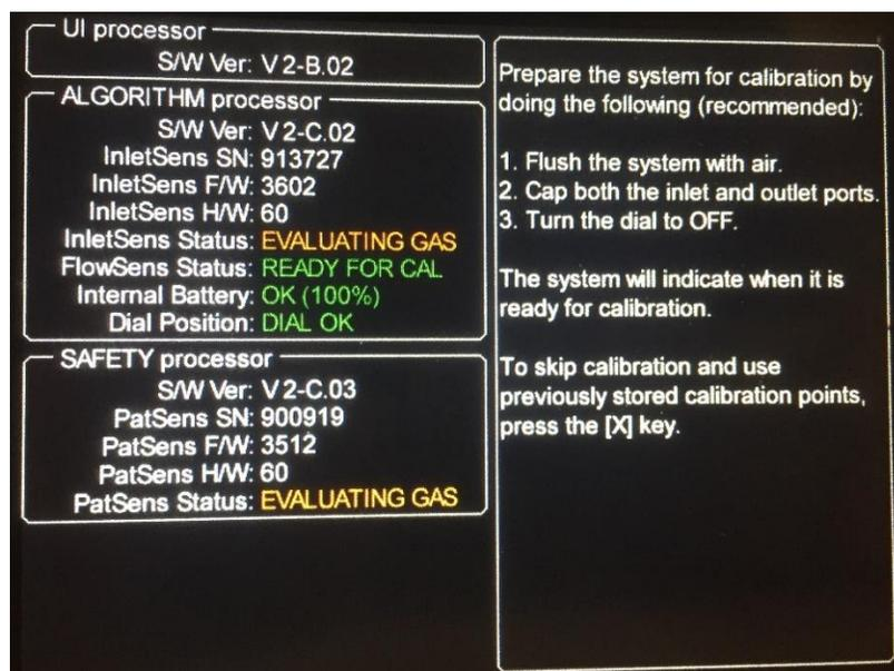
Figure 4: Startup Screen - Preparing for Self-Check
