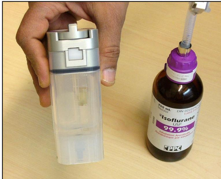
Figure 33: Residual Anesthetic Should Be Drained
