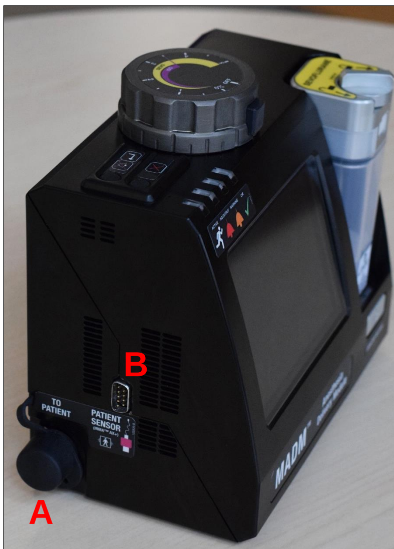
Figure 16: Left Side Connections
