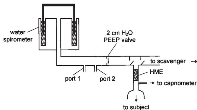
Figure 1. Schematic diagram of breathing circuit. Fresh gas was delivered via port 1 and inspired gas was sampled for CO analysis via port 2. The 2 cm  $H_2O$  PEEP valve prevented fresh gas from escaping into the expiratory limb of the circuit during expiration. HME = heat moisture exchanger.
